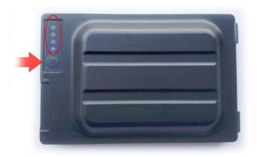
Note: There is a button and four LEDs on the battery. The LEDs will indicate battery capacity when you give the button a short press.
