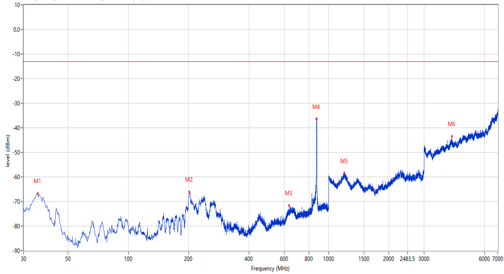
RSE Test case_CE FCC FCC PART22&24&27 FCC PART 22_850_GSM 850&CDMA BC0&WCDMA B5&LTE B5&26
