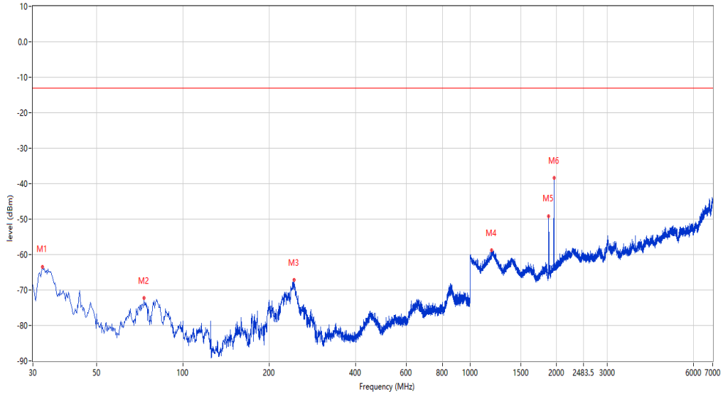
RSE Test case_CE FCC FCC PART22&24&27_FCC PART 24_1900_GSM 1900&WCDMA B2&CDMA BC1&LTE B2
