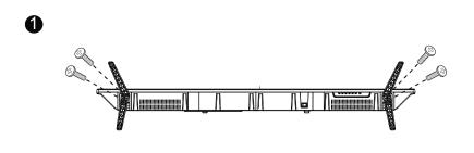
Insert 4 screws M4X12 (provided) through the holes in the bottom of the base into the post holes and tighten securely. Do not over-tighten.
