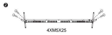
Insert 4 screws M5X25 (provided) through the holes in the bottom of the column and tighten securely. Do not over-tighten.
