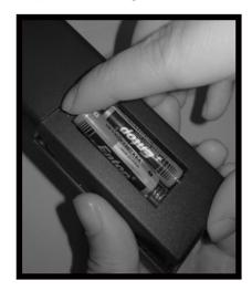
• Place two (2) "AAA" batteries into the battery compartment with the "+" and "-" ends facing as indicated.
