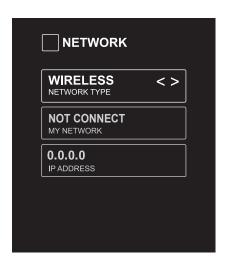
Press MENU to display the main interface, use the Arrow buttons to highlight TV SETTINGS and press OK to confirm. Then Use the Arrow buttons to select NETWORK to enter and adjust each option setting.
