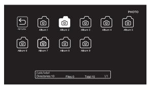
Use the Arrow buttons to highlight the PHOTOS option and press OK, then it will jump to confirm the inserted drive, press OK to enter. After entering PHOTOS, use the Arrow buttons to select the picture file and press OK to enter.
