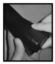
• Turn the remote over and remove battery cover.
