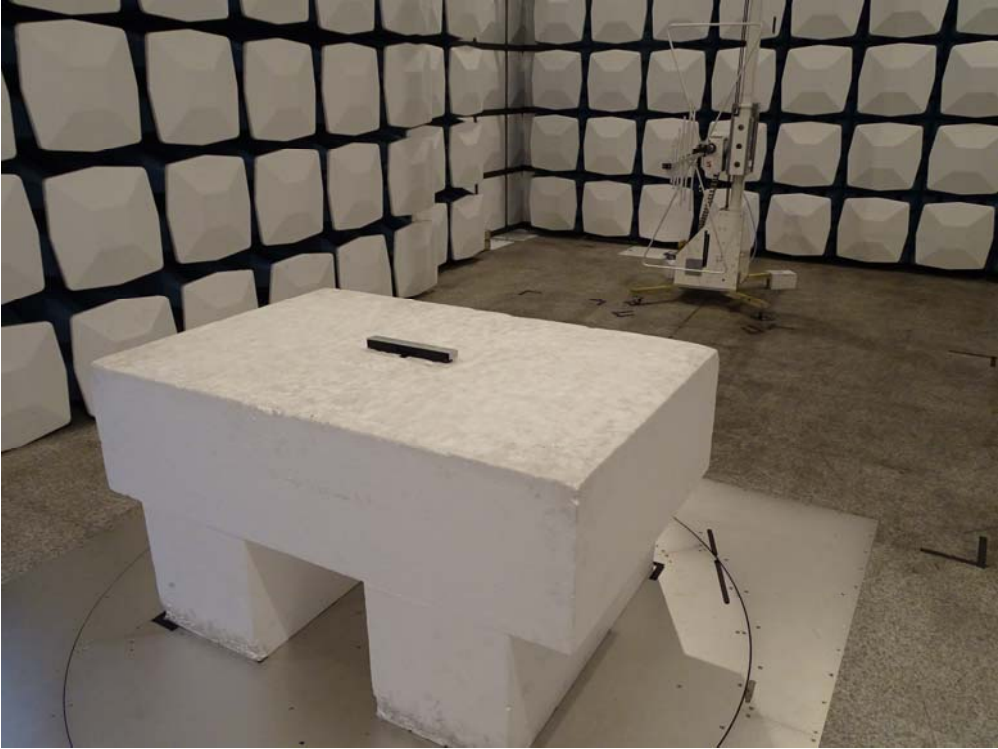
Front View of Spurious Emission Test
