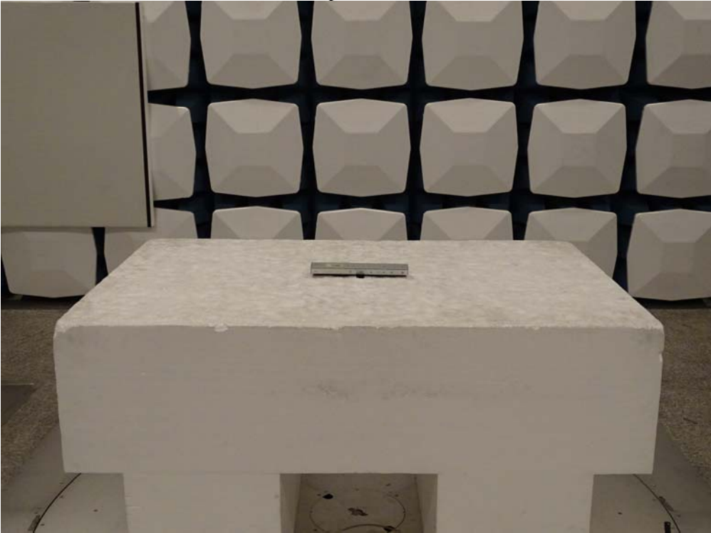
Back View of Spurious Emission Test
