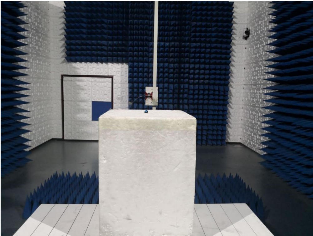
RADIATED EMISSION TEST SETUP ABOVE 1GHZ
