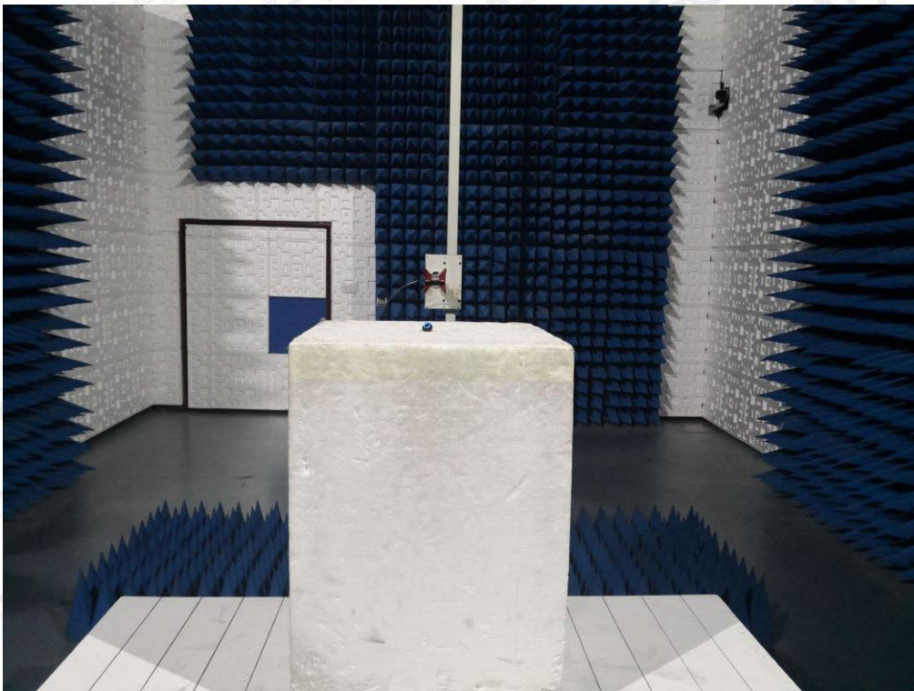
RADIATED EMISSION TEST SETUP ABOVE 1GHZ
