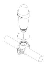
Slightly and slowly unscrew the **Blue Connect** (maximum ½ turn) to remove any air. As soon as the water comes out, it means that there is no air left in the pipes, and you can then tightly screw **Blue Connect** again.
