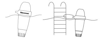
**Note**: Make sure the device is in vertical position and the top part out of the water to allow a correct communication.
