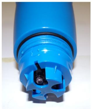
Foot cover removed (Measuring probe view)
