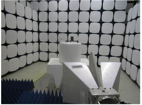
1.3 Radiated Spurious Emissions Test Setup
