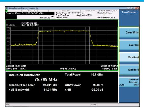
Emission Bandwidth&99% Occupied Bandwidth UNII Band III Test Model 802.11ac(VHT80) mode Frequency(MHz) Ant1
