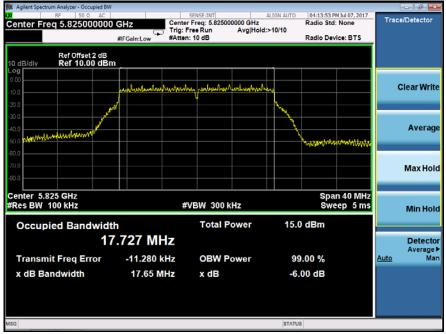
Minimum Emission Bandwidth Test Model 802.11n(VHT40) mode Ant1 UNII Band III Frequency(MHz)
