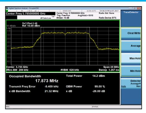
UNII Band III Emission Bandwidth&99% Occupied Bandwidth Test Model 802.11n(VHT20) mode Frequency(MHz)
