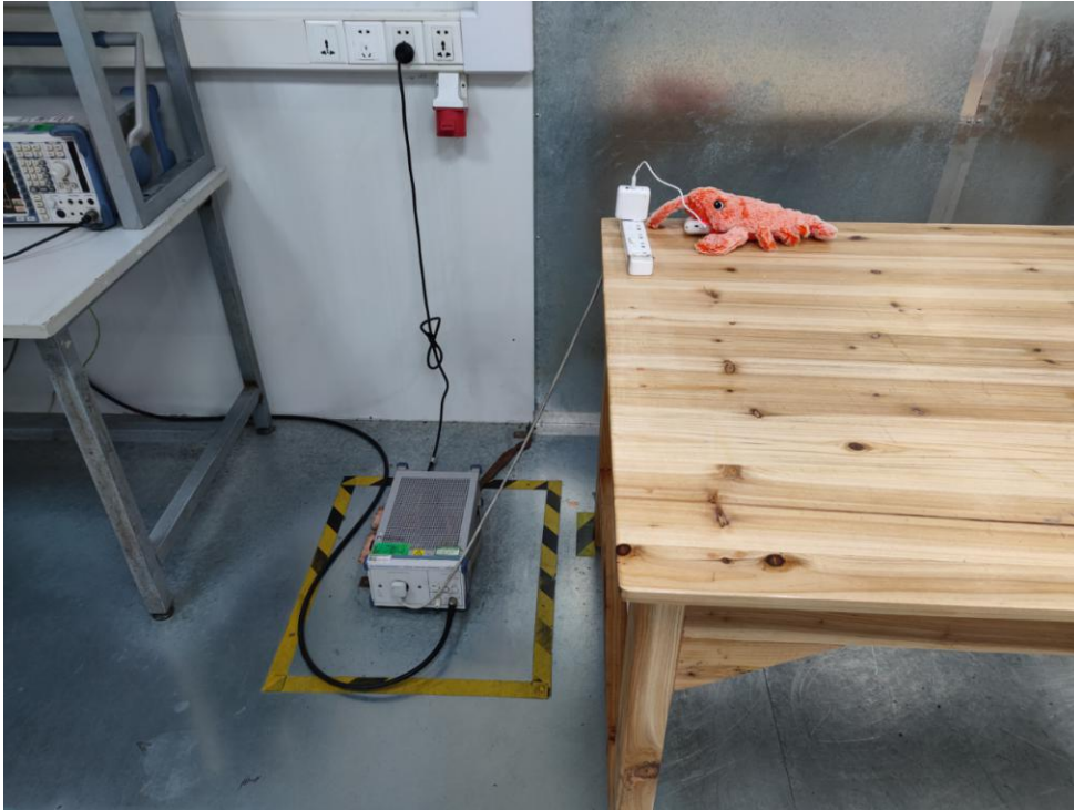
Photo of Conducted Emission Test
