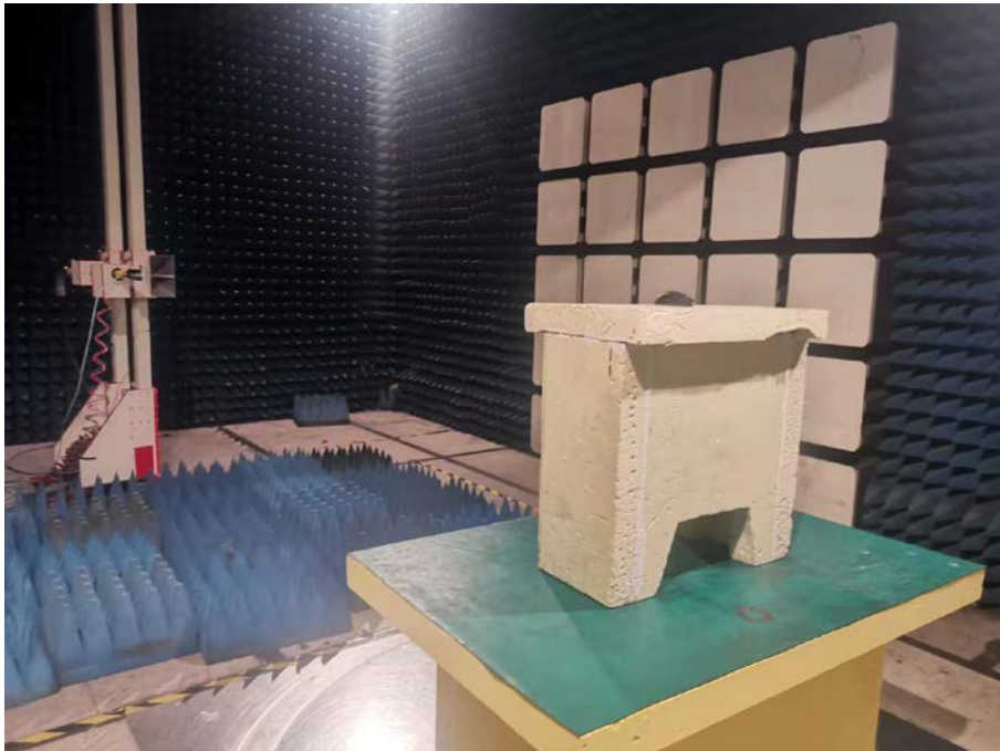
Spurious Emission Test Setup (Above 1GHz)
