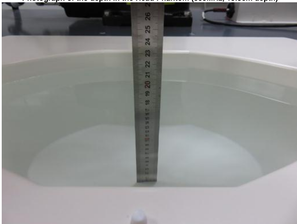
Photograph of the depth in the Body Phantom (1900MHz, 15.9cm depth)
