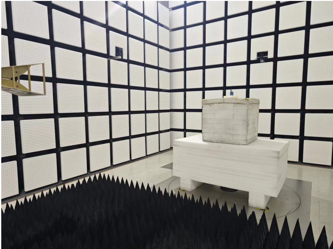
Radiated Emission Above 1GHz View
