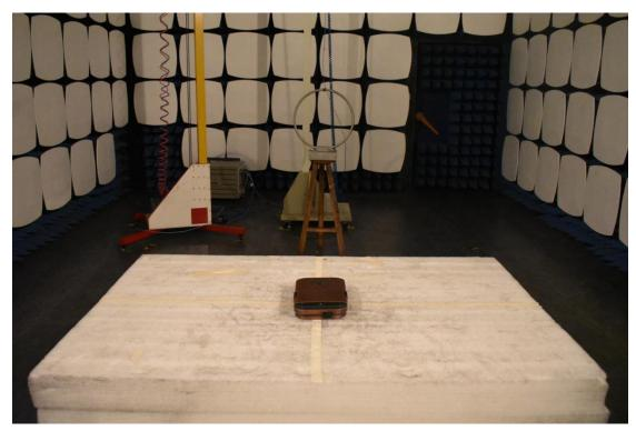
3. Radiated emission (9KHz-30MHz)
