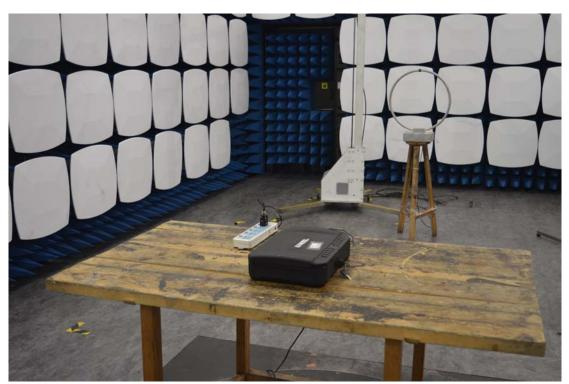
3. Radiated emission (9KHz-30MHz)
