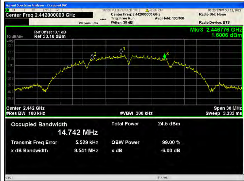
-6dB Bandwidth NVNT b 2442MHz Ant1
