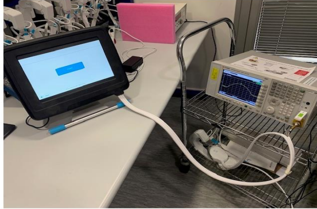
Photograph 3.1.1 Power measurements test setup
