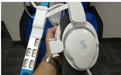
Figure 80: Station selector is disconnected. The separator is between the sensors
