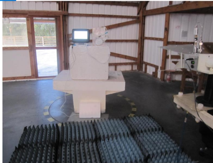
Photograph No.4 Setup for spurious emission field strength measurements at the OATS above 1000 MHz
