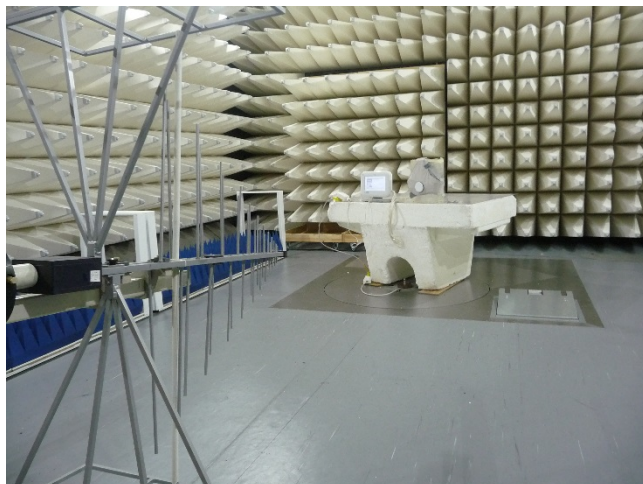
Photograph 8.1.1 Setup for radiated emission measurements
