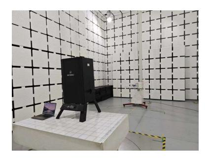
Set-up for Radiated Spurious Emission, Above 1GHz
