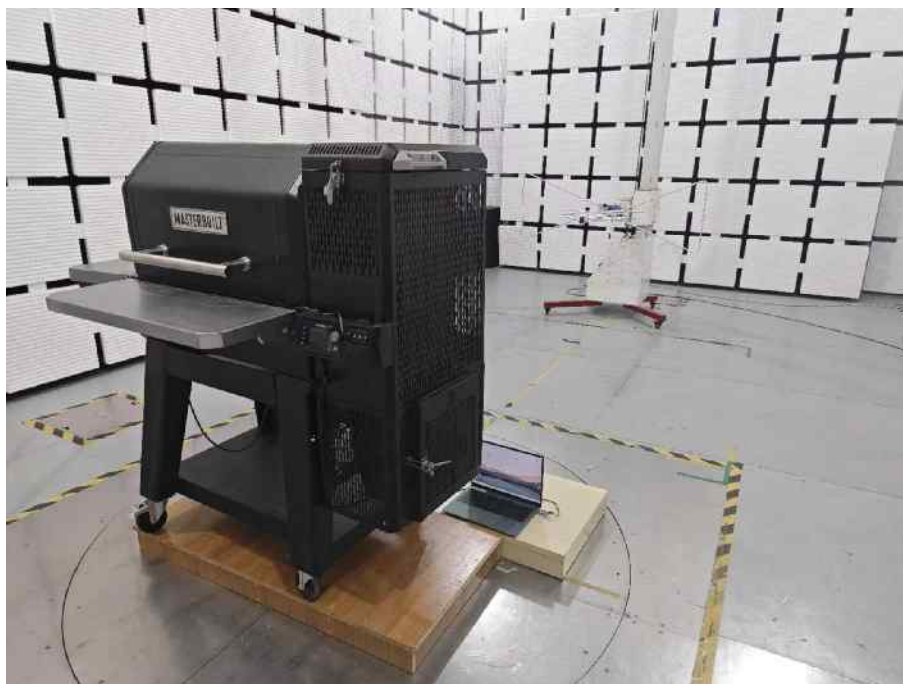
Set-up for Radiated Spurious Emission, Above 1GHz
