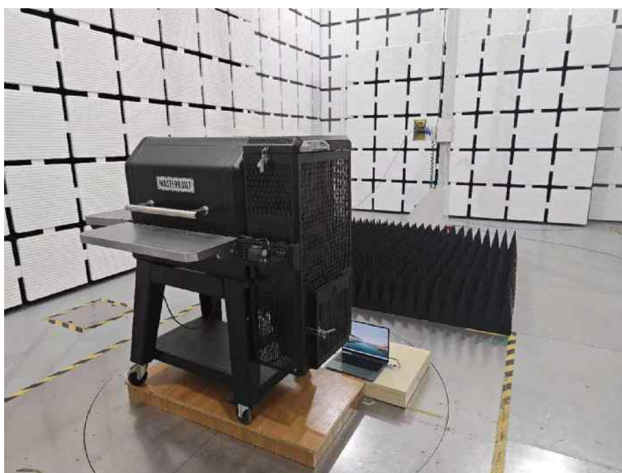
Set-up for Radiated Spurious Emission, Above 1GHz
