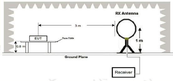
2. Radiated Emission Test-Up Frequency 30MHz~1GHz
