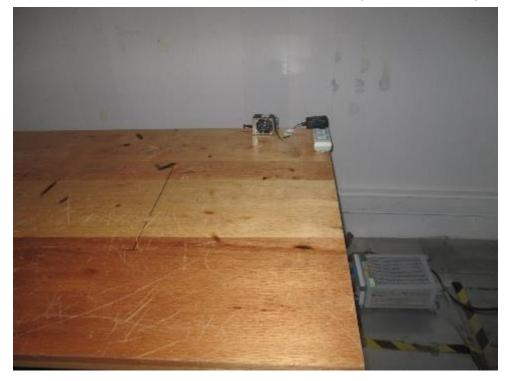
**1.2** Radiated Spurious Emissions Test Setup
