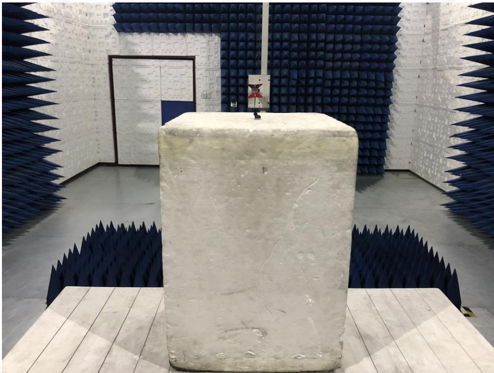
RADIATED EMISSION TEST SETUP ABOVE 1GHZ
