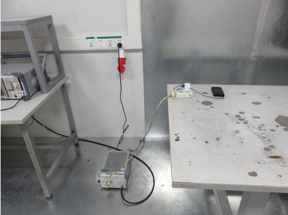
Photo of Conducted Emission Measurement
