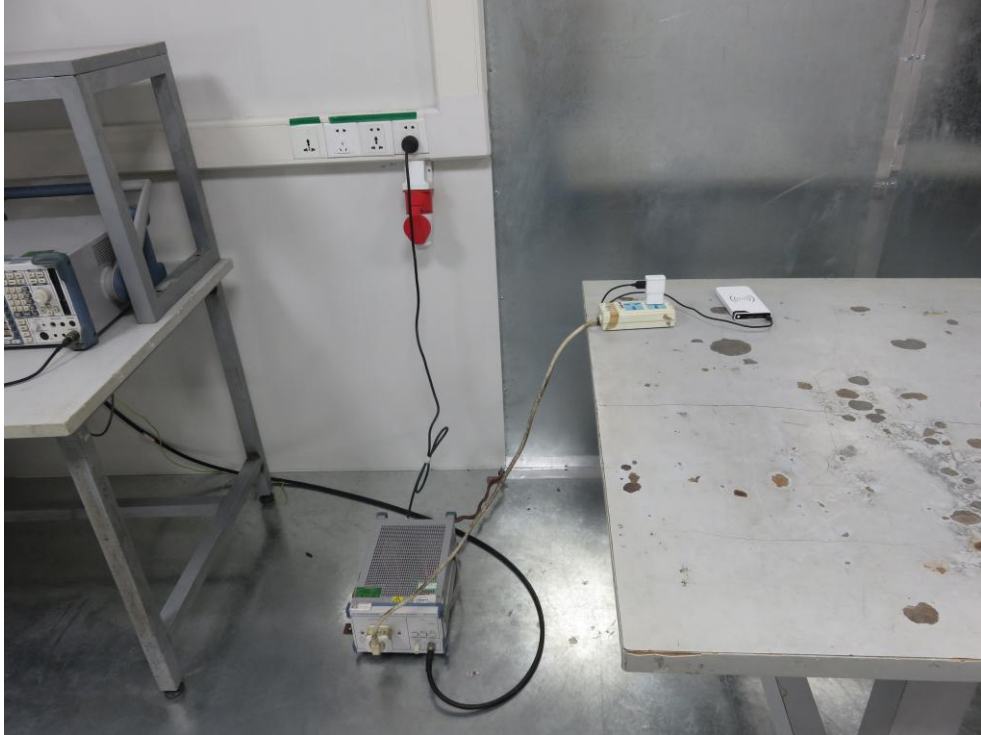
Photo of Conducted Emission Measurement
