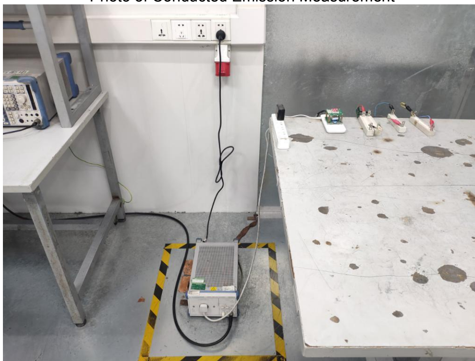
FCC ID: 2AONA-WX1910APD Photo of Conducted Emission Measurement
