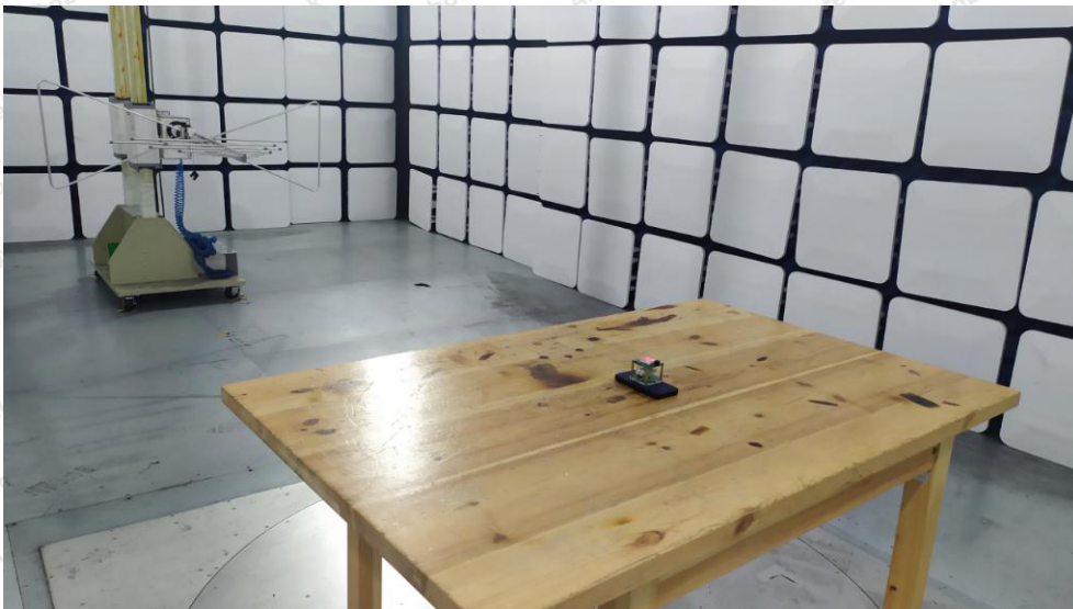
Photo of Radiation Emission Test
