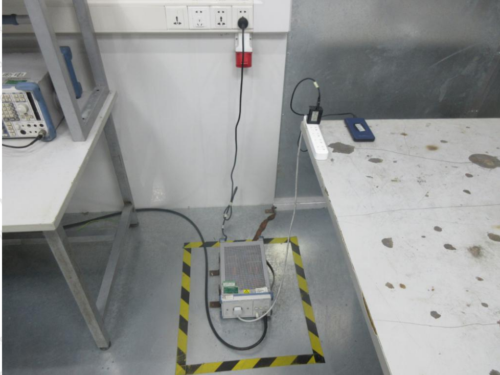
Photo of Conducted Emission Measurement
