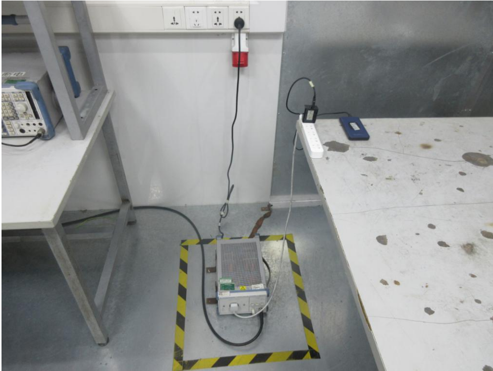
Photo of Conducted Emission Measurement
