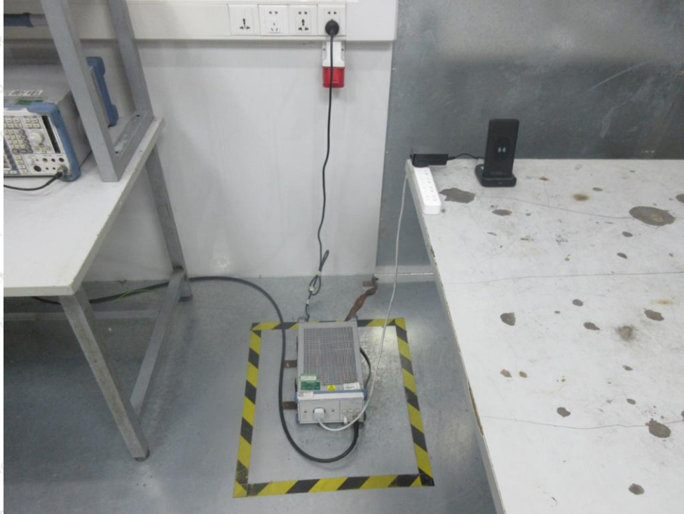
Photo of Conducted Emission Measurement
