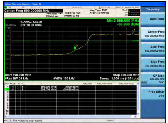
Band12 / 5MHz / Low CH / QPSK / FULL RB
