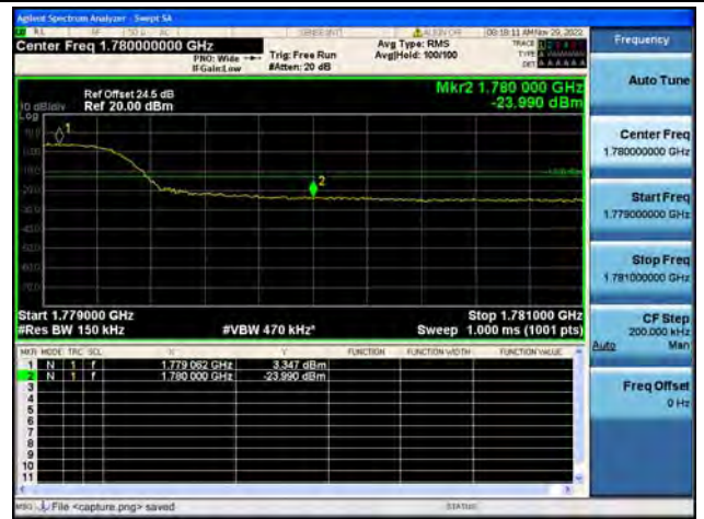
Band66 / 15MHz / High CH / QPSK / FULL RB
