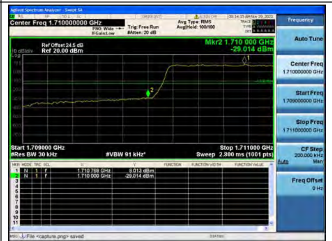
Band66 / 1.4MHz / Low CH / QPSK / FULL RB
