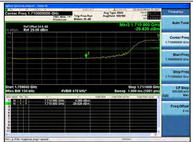
Band4 / 15MHz / Low CH / QPSK / FULL RB
