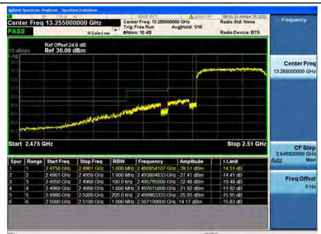
Band7 / 10MHz / Low CH / QPSK / FULL RB
