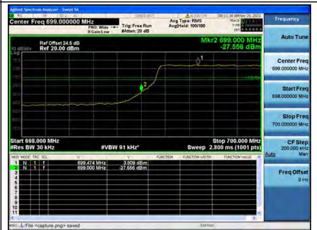
Band12 / 3MHz / Low CH / QPSK / FULL RB
