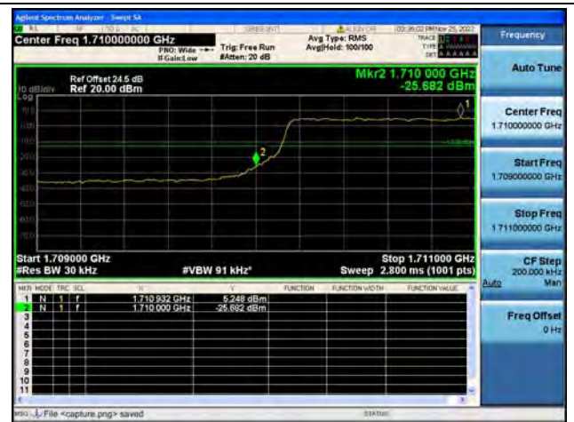
Band4 / 3MHz / Low CH / QPSK / FULL RB
