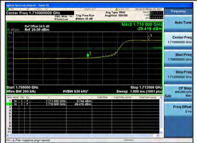
Band4 / 20MHz / Low CH / QPSK / FULL RB
