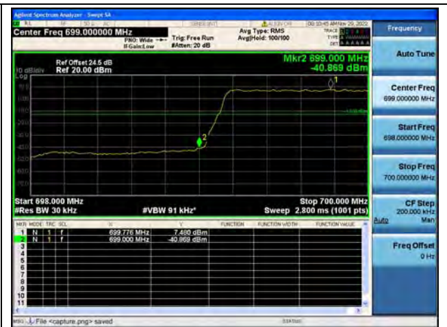
Band12 / 1.4MHz / Low CH / QPSK / FULL RB
