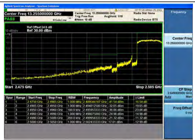
Band7 / 5MHz / Low CH / QPSK / FULL RB
