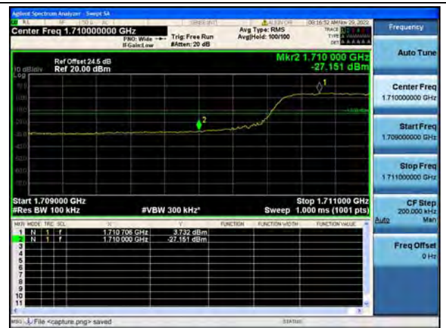
Band66 / 10MHz / Low CH / QPSK / FULL RB
