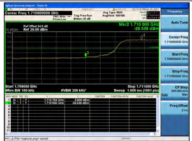
Band4 / 10MHz / Low CH / QPSK / FULL RB
