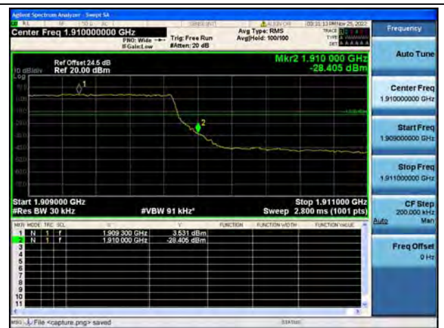
Band2 / 3MHz / High CH / QPSK / FULL RB
