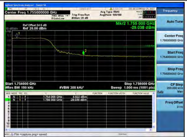
Band4 / 10MHz / High CH / QPSK / FULL RB
