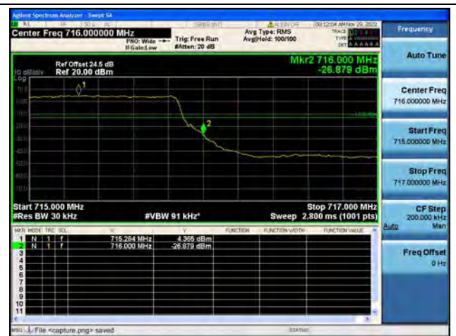
Band12 / 3MHz / High CH / QPSK / FULL RB
