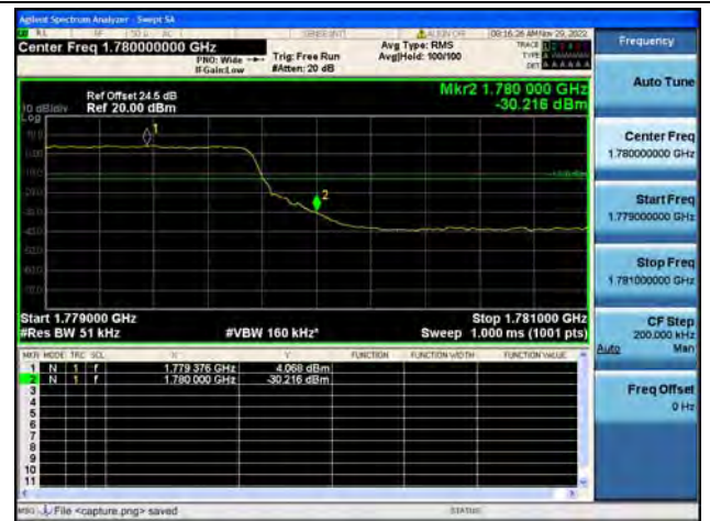
Band66 / 5MHz / High CH / QPSK / FULL RB
