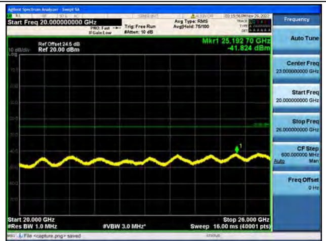
Band7-20G-26G / 20MHz / Low CH / QPSK
