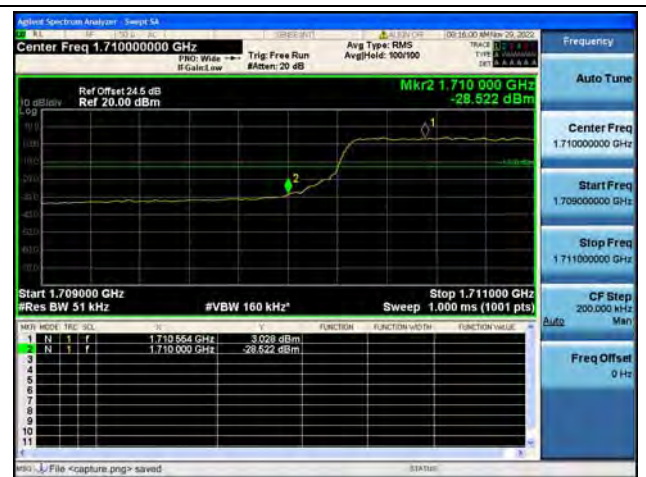
Band66 / 5MHz / Low CH / QPSK / FULL RB
