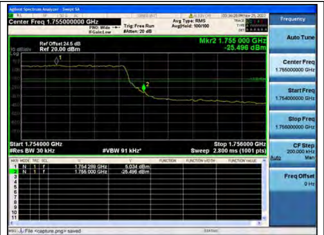
Band4 / 3MHz / High CH / QPSK / FULL RB
