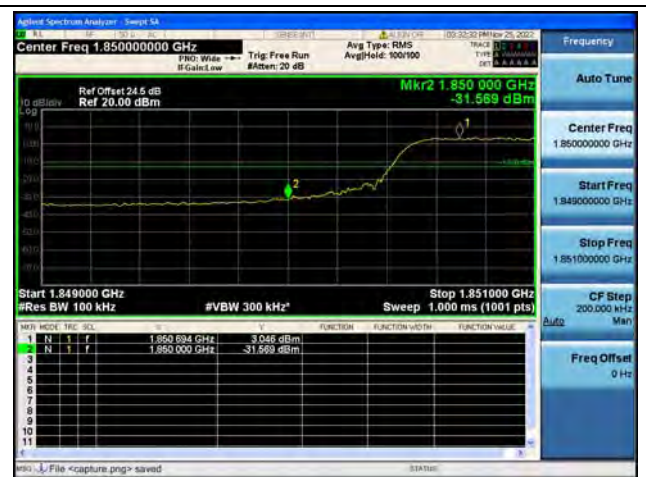
Band2 / 10MHz / Low CH / QPSK / FULL RB
