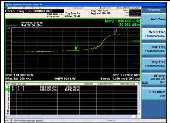
Band2 / 20MHz / Low CH / QPSK / FULL RB
