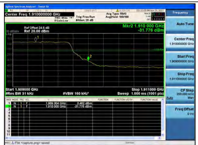
Band2 / 5MHz / High CH / QPSK / FULL RB
