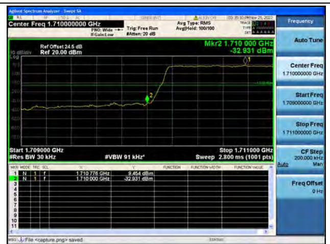
Band4 / 1.4MHz / Low CH / QPSK / FULL RB
