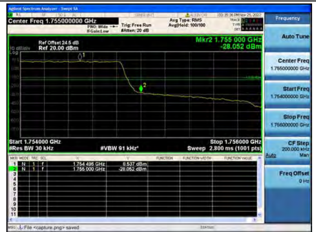
Band4 / 1.4MHz / High CH / QPSK / FULL RB
