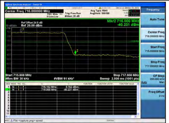
Band12 / 1.4MHz / High CH / QPSK / FULL RB
