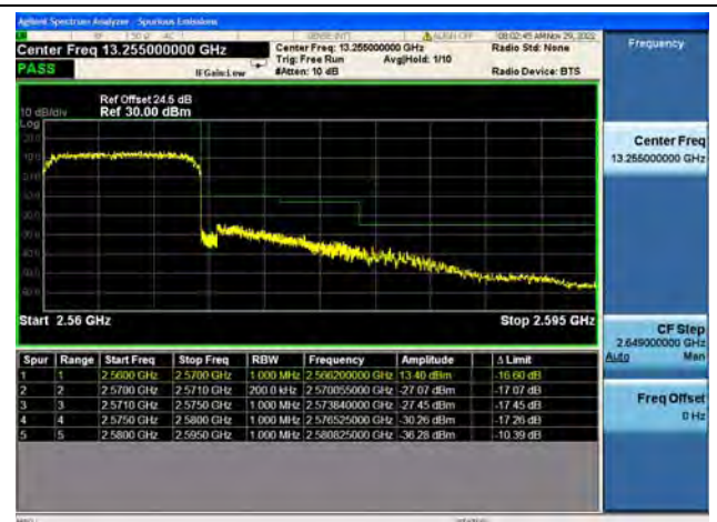
Band7 / 10MHz / High CH / QPSK / FULL RB
