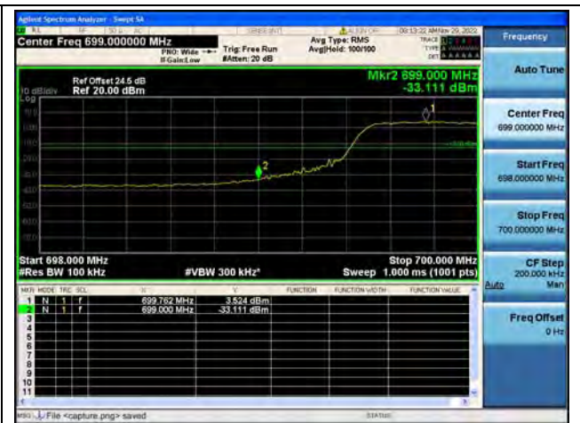
Band12 / 10MHz / Low CH / QPSK / FULL RB
