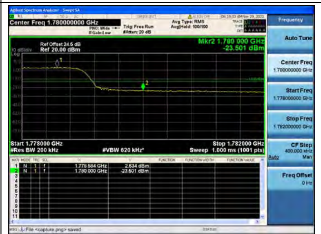
Band66 / 20MHz / High CH / QPSK / FULL RB
