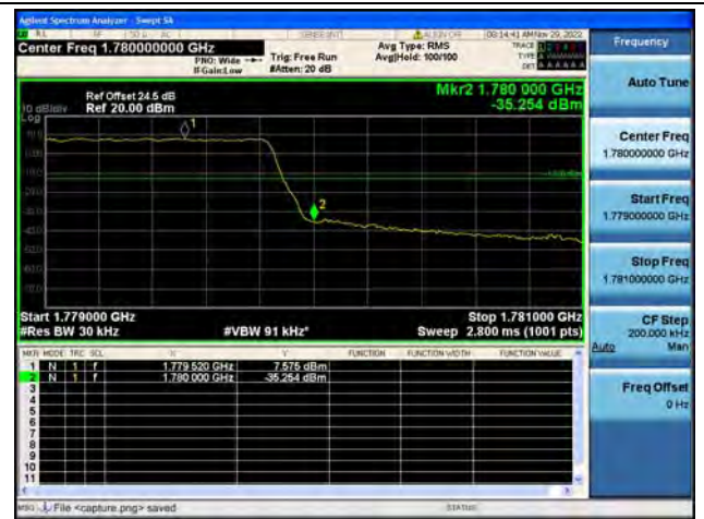
Band66 / 1.4MHz / High CH / QPSK / FULL RB
