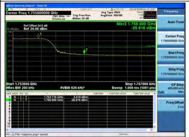
Band4 / 20MHz / High CH / QPSK / FULL RB
