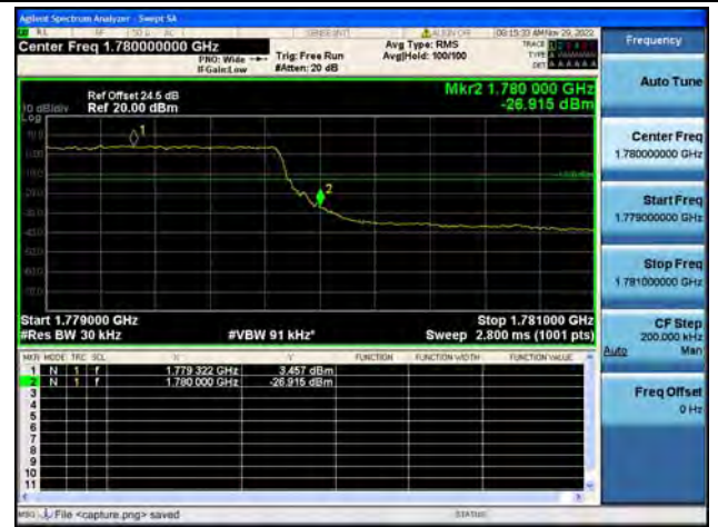
Band66 / 3MHz / High CH / QPSK / FULL RB
