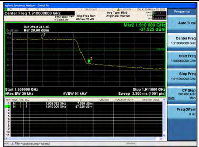
Band2 / 1.4MHz / High CH / QPSK / FULL RB
