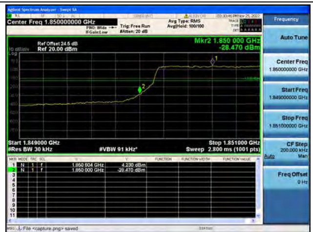
Band2 / 3MHz / Low CH / QPSK / FULL RB
