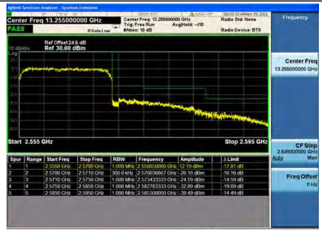
Band7 / 15MHz / High CH / QPSK / FULL RB
