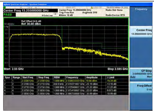
Band7 / 20MHz / High CH / QPSK / FULL RB
