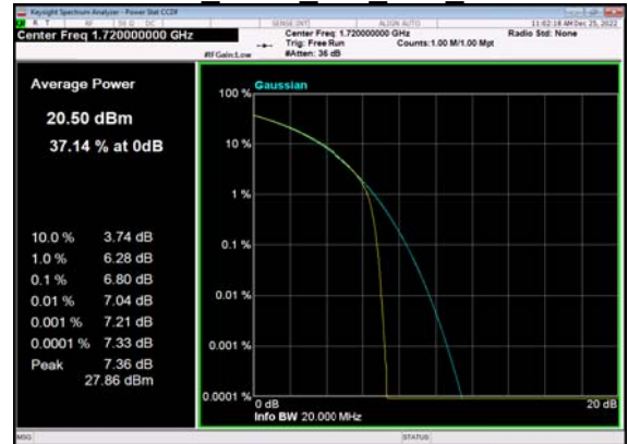
N66(20M)_CP-OFDM_16 QAM Outer Full Low CH
