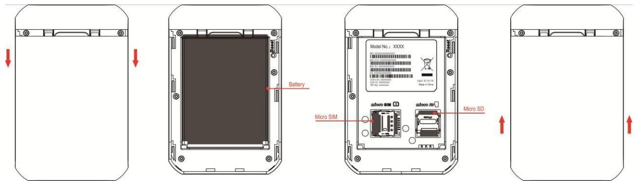
Tips: Always switch the device off and disconnect the charger before removing the battery.
