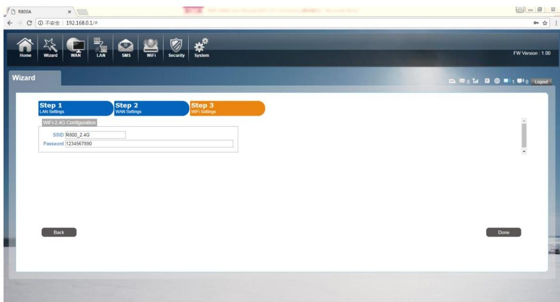
You can quickly change the LA configuration, set the APN, and change the 2.4G SSID/Password through the wizard function.
