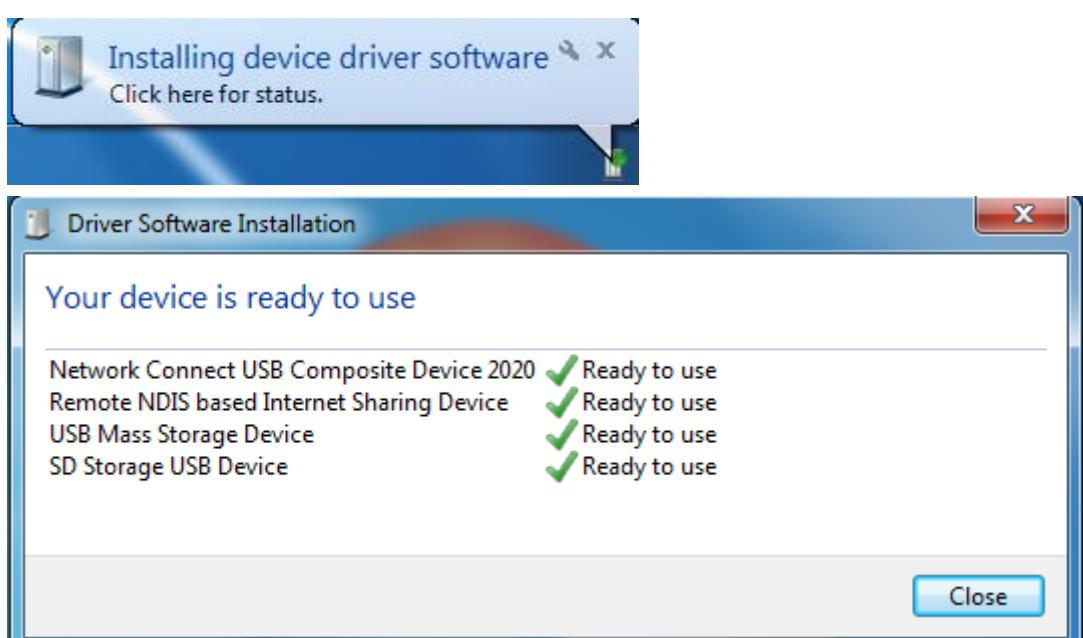
3. Check the network card is installed correctly, like the following pictures
