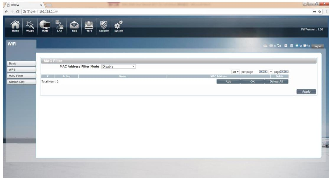
Deny list Stations: If you add the computers or wireless devices MAC address into the list, it can prohibiting the computers or wireless devices connect to the R800C. The computes or wireless devices MAC address which are not in the list can able to connect to R800C.
