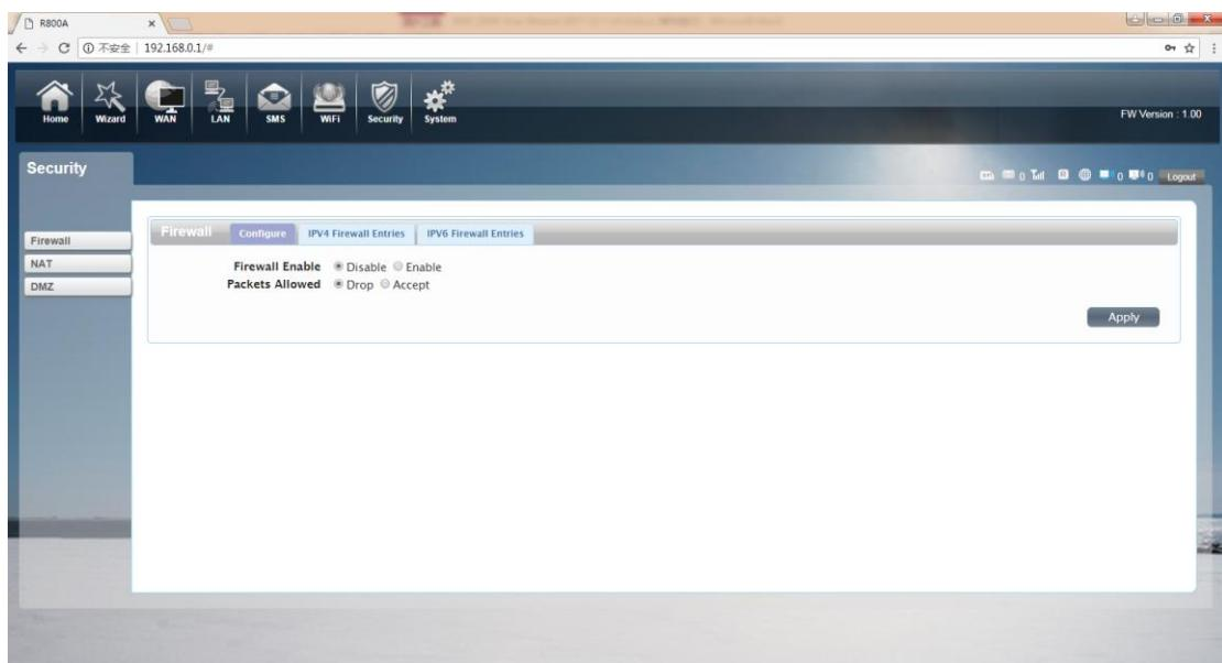
Firewall configuration: You can Disable or Enable the Firewall function. Also you can setting the matching packets rule to receive or reject.
