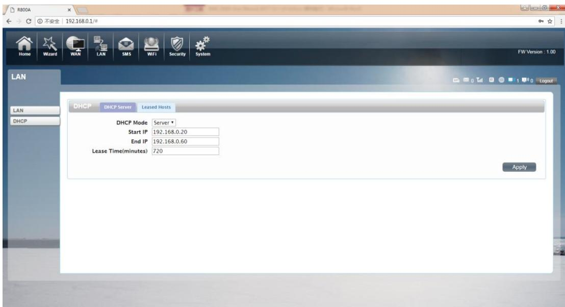
DHCP Mode: Select the server mode, the device can be done using a DHCP server; choose none, which is off the server function.
