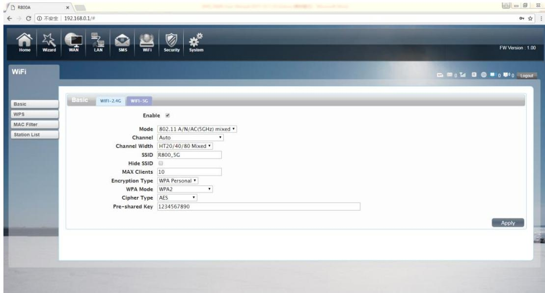
★Recommend that you start using R800C administration pages after setting a convenient landing memorizing SSID and a higher safety factor Wi-Fi passwords
