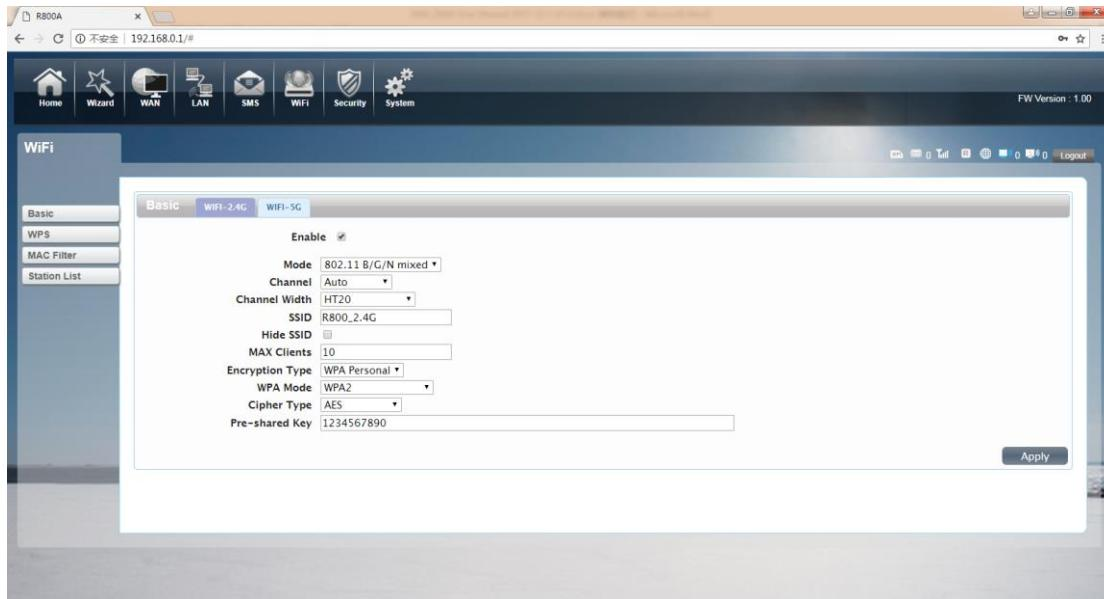
We can setting the 2.4G WiFi configuration in this page, like B/G/N mode, Channel,
