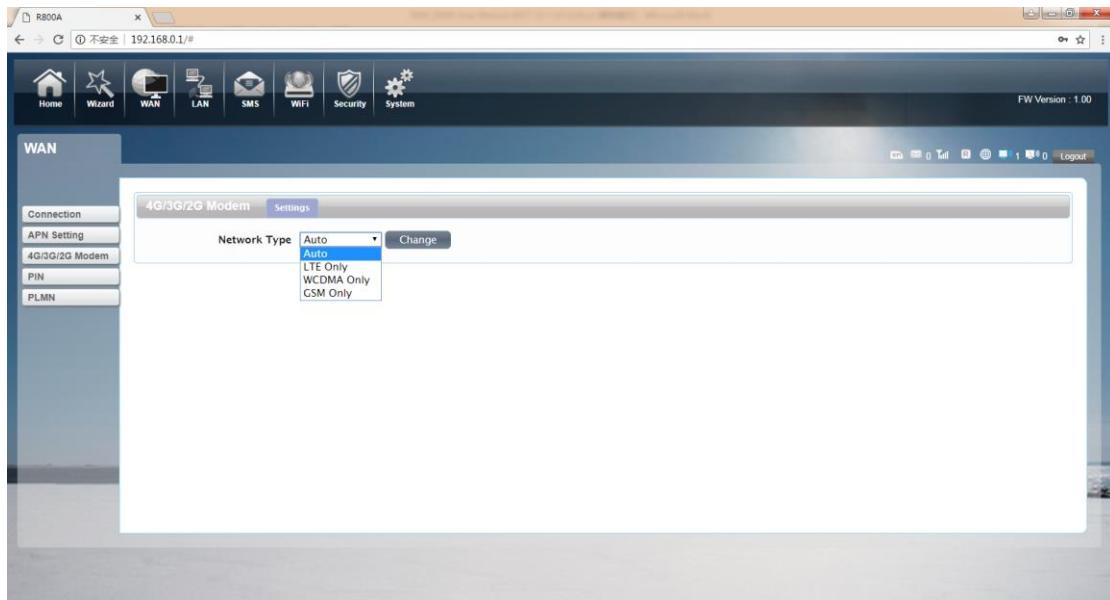
There are four types of networks can be choose: Auto is 4G/3G/2G, Leanly is using only 4G, WCDMA Only is using only 3G,GSM Only is using only 2G.
