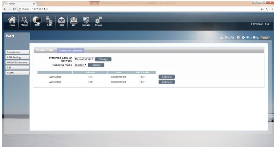
**2. APN Setting:** You can customize the network configuration or manually add the new APN and set defaulting.
