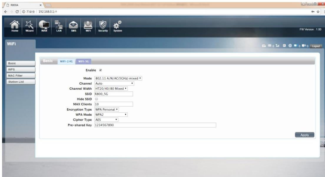
You can also control the opening and closing of 5G WiFi, and set up the WiFi Channel .The 5G WiFi of R800C supports 802.11 A/N/AC Mixed protocol. We set the Channel Width to reach HT20/40/80 Mixed. The highest 5GWIFI rate can reach
