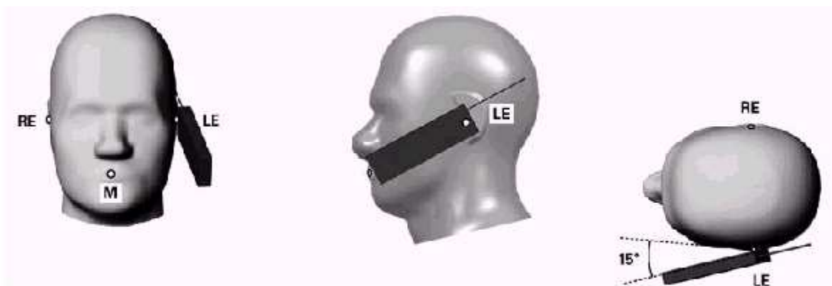
Figure 3 Tilt position of the wireless device on the left side of SAM
