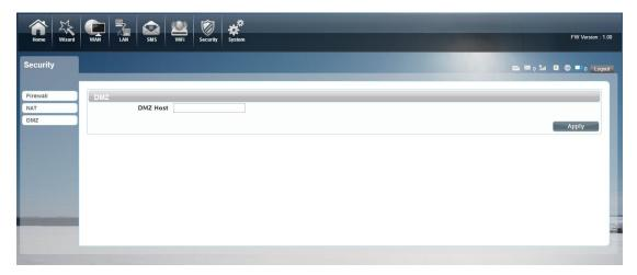
Receive all the data from external network interface forwarded to "DMZ IP address" Enable DMZ: If an application has trouble working from behind the router, you can expose one computer to the Internet and run the application on that computer.
