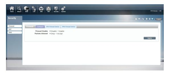
Firewall configuration: You can Disable or Enable the Firewall function. Also you can setting the matching packets ipv6/ipv4 rule to receive or reject.
