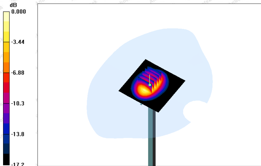
System Performance Check 1900MHz Head 250mW
