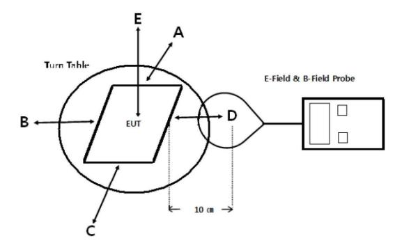
Note: Measurements should be made from all sides and the top of the primary/client pair, with the 10cm measured from the center of the probe(s) to the edge of the device.
