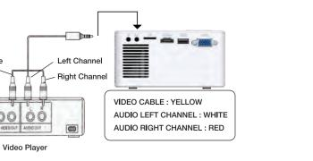
Follow the diagram below to connect the GOTheater to a device that has RCA
