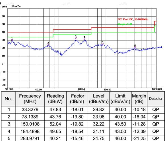
1). Emission level  $(dBuV/m) = 20 \log Emission level (uV/m)$ .
