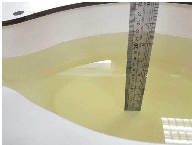
Photograph of the depth in the Head Phantom (1900MHz, 15.1cm depth)
