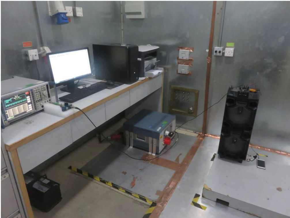
FCC RADIATED EMISSION TEST SETUP
