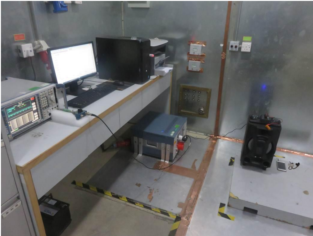
FCC RADIATED EMISSION TEST SETUP
