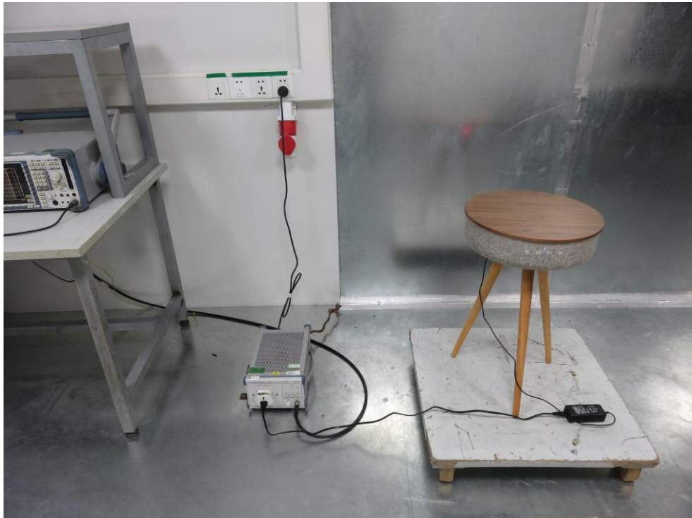
Photo of Conducted Emission Test
