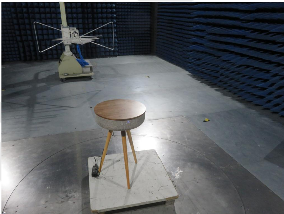
Photo of Radiation Emission Test
