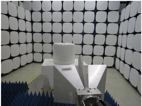
1.2 Radiated Spurious Emissions Test Setup
