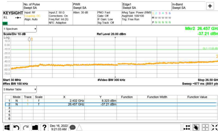
Right, Conducted Spurious Emissions, \pi/4 DQPSK, Middle Channel (2 440 MHz)
