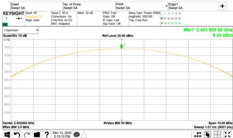
Left, Maximum Peak Output Power, GFSK, Lowest Channel
