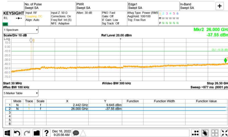
Right, Conducted Spurious Emissions, \pi/4 DQPSK, Middle Channel (2 440 MHz)
