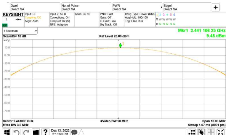
Left, Maximum Peak Output Power, GFSK, Middle Channel
