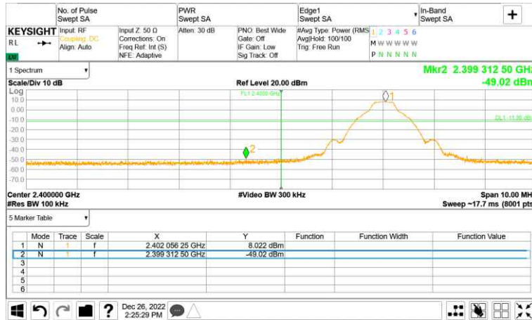
Left, Band Edge, GFSK, Lowest Channel (2 402 MHz)
