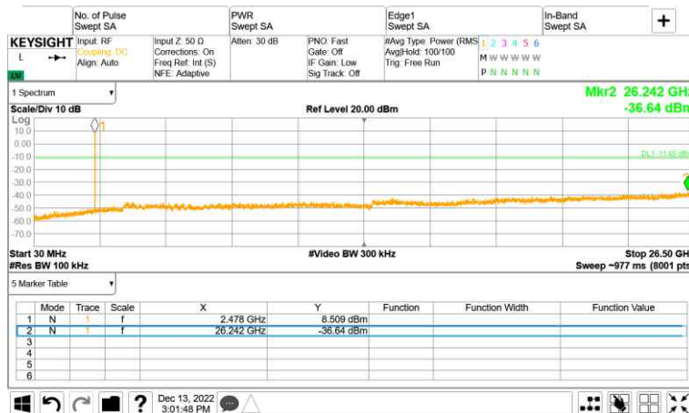
Left, Conducted Spurious Emissions, GFSK, Highest Channel (2 480 MHz)
