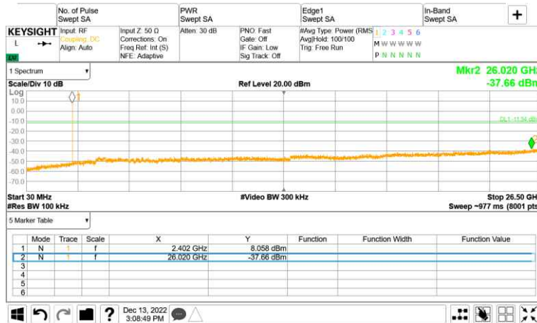
Left, Conducted Spurious Emissions, GFSK, Lowest Channel (2 402 MHz)
